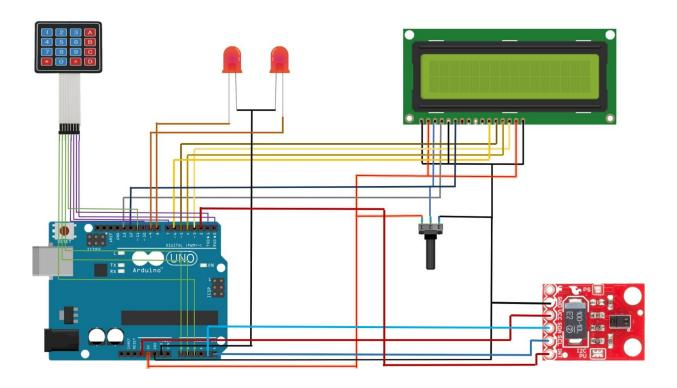
The gesture sensor, and the LCD module are interfaced with the Arduino board. The Arduino UNO controls and operates the different interfaced sensors, and modules. The circuit connections are as follows –
